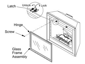
Figure 37 - Removing/Replacing Glass Door
